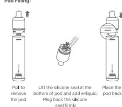
• When you place the pod back, make sure that the buckle is aligned with the position of the airflow hole.
